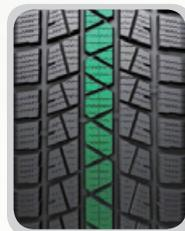
Central rib pattern and multi-sipe design makes excellent braking and steering performance on snow/ice terrain.
